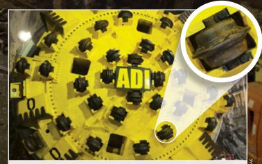
**Cut!** The TBM features a 22-foot-tall, 200-ton cutter head with 44 rotating steel disks that workers change every two to three weeks.
